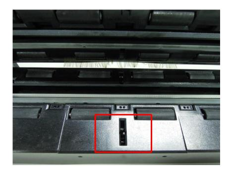
When the scanner is power on, user inserts the paper from the front end, if the Sensor1 detects the paper, the VTM 300 will feed the paper. At the same time, the VTM 300 will detect the skew and the paper jam, if there is no abnormal situation, the VTM 300 will feed the paper.
